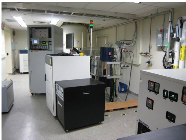
395 GHz/600 MHz DNP-NMR spectrometer, the University of Guelph NMR Centre
