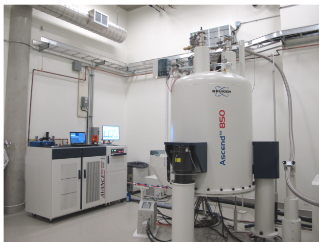
The 850 MHz NMR spectrometer in the basement of the Life Sciences Centre.
