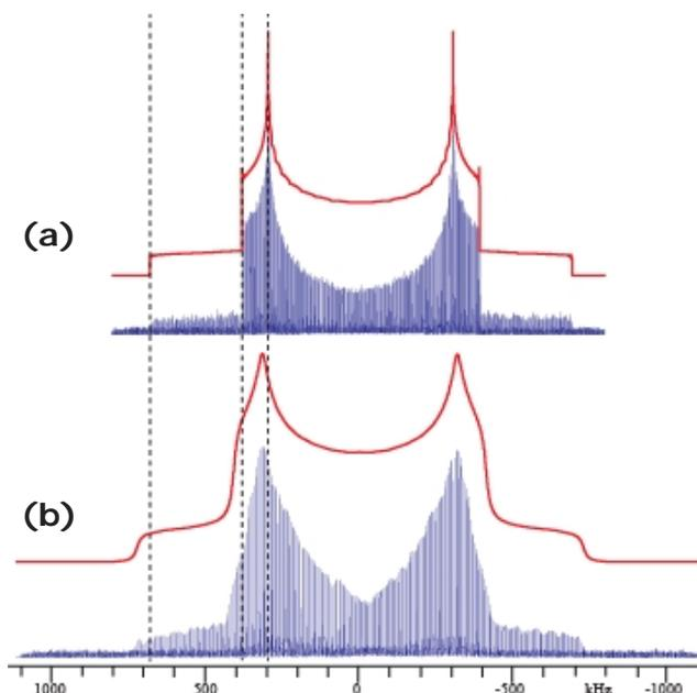
**Figure 2:**  $^{14}\text{N}$  powder patterns of (a) mexil I,  $C_Q = 0.915$  MHz and  $\eta_Q = 0.125$  and (b) mexil III,  $C_Q = 0.97$  MHz and  $\eta_Q = 0.13$ . The spectra recorded at 21.1 T are composed of 2 and 4 sub-spectra, respectively, and took ca. 2 and 5 hours, respectively, to collect. Dashed vertical lines highlight discontinuities of mexil I.
