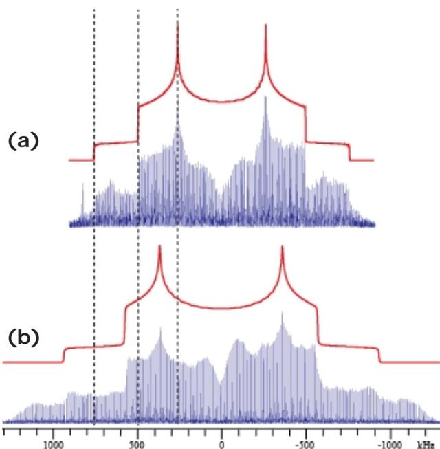
**Figure 1:**  $^{14}\text{N}$  powder patterns of (a) bupiv I,  $C_Q = 1.00$  MHz and  $\eta_Q = 0.31$  and (b) bupiv II,  $C_Q = 1.25$  MHz and  $\eta_Q = 0.22$ . The spectra taken at 21.1 T are composed of 2 and 4 sub-spectra, respectively, and took ca. 8 and 16 hours, respectively, to collect. Dashed lines highlight discontinuities of bupiv I.
